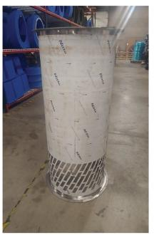
2. Once the intake section is completely positioned properly, install foam tape on top ring of intake section
