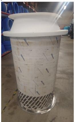
4. Apply foam tape to the top of the vertical poly blank. Attach elbow assembly using four (4)  $1\&\frac{1}{2}$ " stainless steel bolts, eight (8) stainless steel fender washers and four (4) stainless steel nuts. Lift the entire section and place it on top of the intake section. Secure using four (4)  $1\&\frac{1}{2}$ " stainless steel bolts, eight (8) stainless steel fender washers and four (4) stainless steel nuts.
