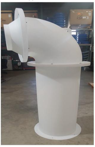
6. Raise and attach horizontal and elbow (with hogger) to the attached poly vertical blank using four (4)  $1\&\frac{1}{2}$ " stainless steel bolts, eight (8) stainless steel fender washers and four (4) stainless steel nuts.
