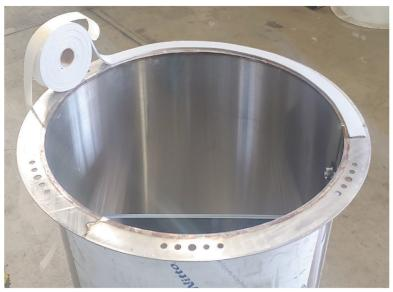
3. Lift up the side nozzle column section and place it on top of the intake section. Bolt in place using four (4)  $1\&\frac{1}{2}$ " stainless steel bolts, eight (8) stainless steel fender washers and four (4) stainless steel nuts. Direct nozzles at approximately a
