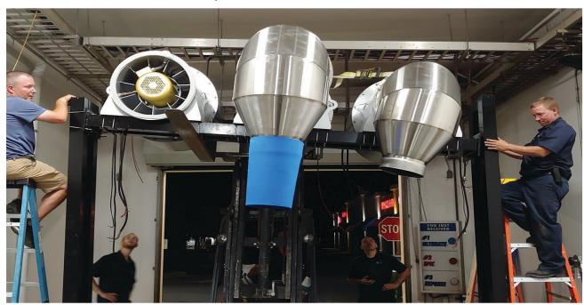
7. If installing a single (1) dual motor, attach 10" blank & second motor on arch.
