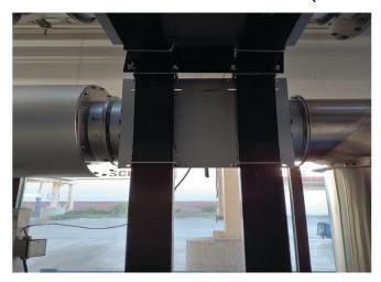
18. Attach the center top nozzle in downward direction using 24" stainless steel extension.
