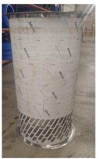
2. Once the intake section is completely positioned properly, install foam tape on top ring of intake section
