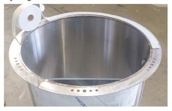
3. Install transition ring on top of intake using four (4) 1&½" stainless steel bolts, eight (8) stainless steel fender washers and four (4) stainless steel nuts. Apply foam tape to the exposed side of poly transition ring.
