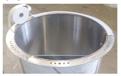
3. Lift up the side nozzle column section and place it on top of the intake section. Bolt in place using four (4) 1&½" stainless steel bolts, eight (8) stainless steel fender washers and four (4) stainless steel nuts. Direct nozzles at approximately a 15 degree angle to the entrance.
