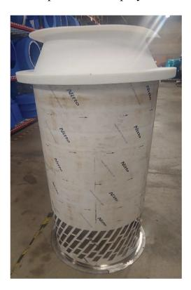
4. Apply foam tape to the top of the vertical poly blank. Attach elbow assembly using four (4)  $1\&\frac{1}{2}$ " stainless steel bolts, eight (8) stainless steel fender washers and four (4) stainless steel nuts. Lift the entire section and place it on top of the intake section. Secure using four (4)  $1\&\frac{1}{2}$ " stainless steel bolts, eight (8) stainless steel fender washers and four (4) stainless steel nuts.
