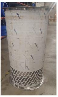
2. Once the intake section is completely positioned properly, install foam tape on top ring of intake section
