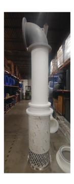
5. Apply foam tape to both ends of poly horizontal blank. Attach elbow to one end using four (4) 1&½" stainless steel bolts, eight (8) stainless steel fender washers and four (4) stainless steel nuts. Apply foam tape to the exposed side of elbow and attach poly hogger using four (4) 1&½" stainless steel bolts, eight (8) stainless steel fender washers and four (4) stainless steel nuts.
