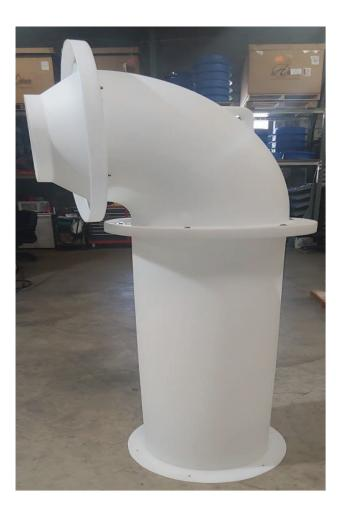
6. Raise and attach horizontal and elbow (with hogger) to the attached poly vertical blank using four (4) 1&½" stainless steel bolts, eight (8) stainless steel fender washers and four (4) stainless steel nuts.
